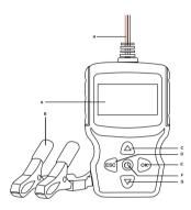
A LCD Display - shows menus, test results and operation tips.
