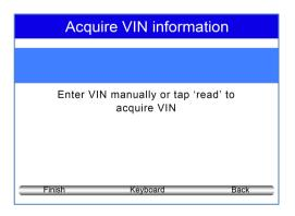
2. Input a valid VIN code and use the function key **Finish** to confirm. The scan tool starts to identify the vehicle.
