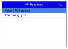
Depending on readiness test, one of these 2 screens will be present. Use the up and down arrow keys to scroll through data. Press the BACK key to exit.
